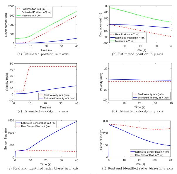
Fig. 11. Estimate radar biases regardless of manoeuvring acceleration.
