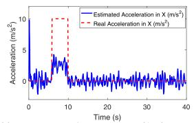
(e) Real and identified acceleration (Avg) in x axis
