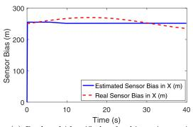
(g) Real and identified radar biases in x axis
