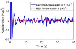
(b) Real and identified acceleration in  $\boldsymbol{y}$  axis
