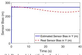
(h) Real and identified radar biases in y axis
